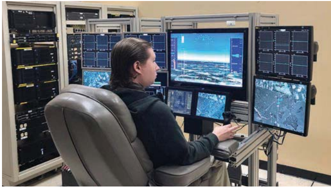
An example of a flight deck style control station with multiple displays that would be operated with a menu structure.
