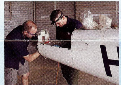
In March, Aaron and Jason repair the aft fuselage of the second plane.
