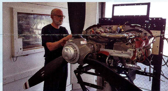
Tim prepares a Continental TSIO-360 for its test run.
